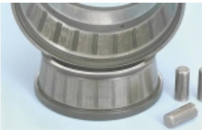
(A-7130)</li> <li>■ Rust on outer ring raceway surface of Tapered Roller Bearing<br/>
