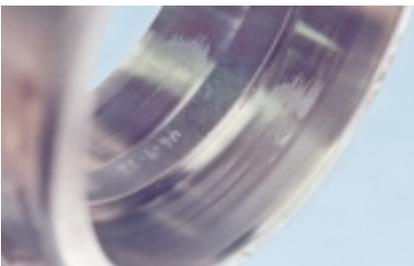
(A-7435)                         </li> <li>Smearing on roller rolling surface of Cylindrical Roller Bearing
