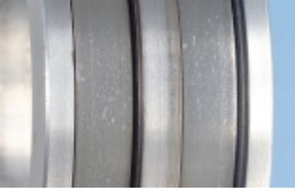
(A-6556)</li> <li>■ Pear skin on inner ring raceway surface of Deep Groove Ball Bearing<br/>
