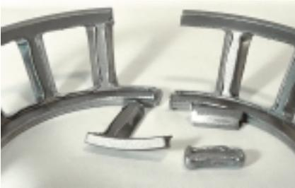
(A-6670)</li> <li>● Distortion of Cylindrical Roller Bearing cage<br/>
