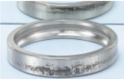
(A-6735)</li> <li>▲ False brinelling on inner ring raceway surface of Deep Groove Ball Bearing<br/>
