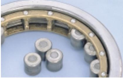
(A-6457)</li> <li>■ <b>Seizure of Cylindrical Roller Bearing with rib</b><br/>
